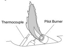
Figure 19 - Incorrect Pilot Flame Pattern
